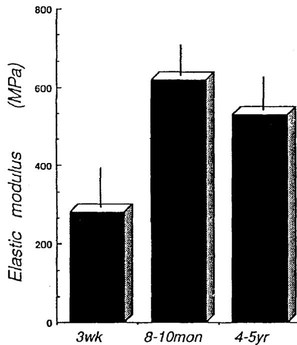
Fig. 7 Changes in the elastic modulus of Achilles tendon during aging. Values are expressed as mean and standard error.
