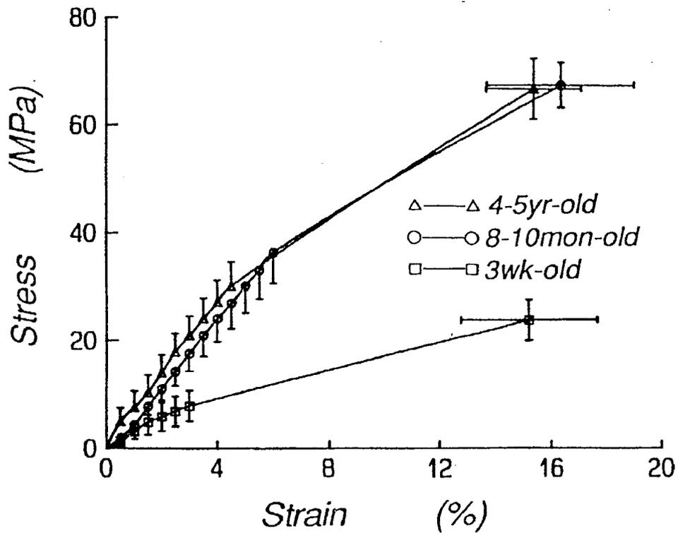
Fig. 2 Stress-strain curves of the mechanical properties of Achilles tendon with aging. Values are expressed as mean and standard error.
