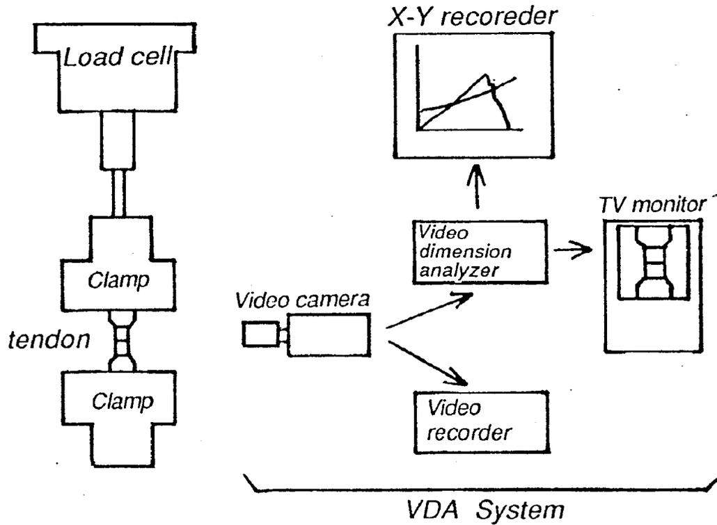
Fig. 1 Experimental apparatus used to determine the mechanical properties of Achilles tendon.
